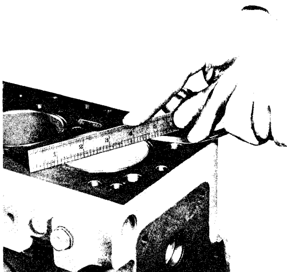
G2 Method of checking Liner protrusion.
